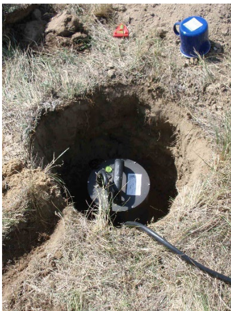
Figure 5: Seismometers are installed in shallow pits.
