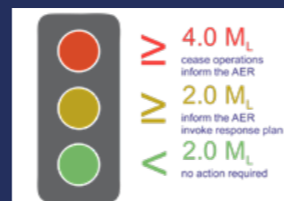
EXAMPLE MONITORING THRESHOLDS FOR TRAFFIC LIGHT SYSTEMS
